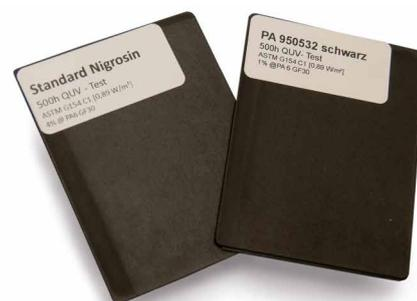
Fig. 3: PA6 GF30 plates, colored with PA 950532 black as compared to a standard nigrosine black according to 500 h QUV tester [ASTM G 154 C1].
